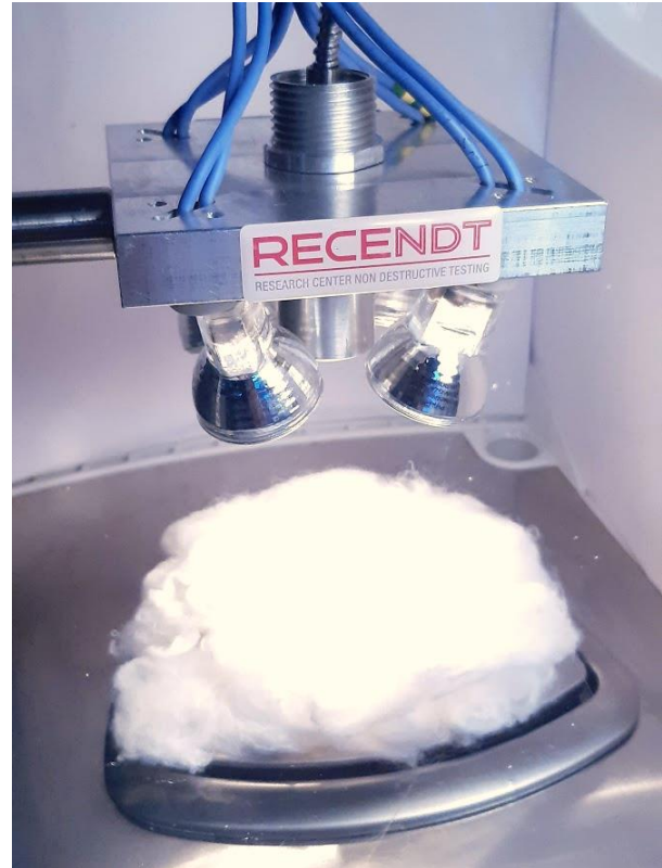
Laboratory setup for moisture determination using near-infrared spectroscopy. © RECENTD GmbH
